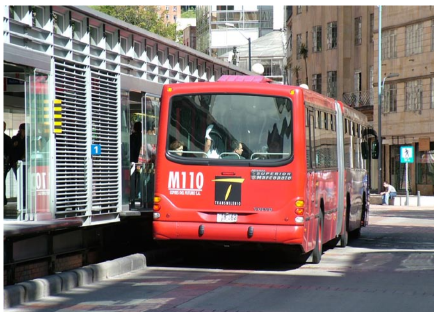
Fig. 35 Segregated bus lanes and rapid boarding facilities at bus stations make the TransMilenio BRT system attractive.
