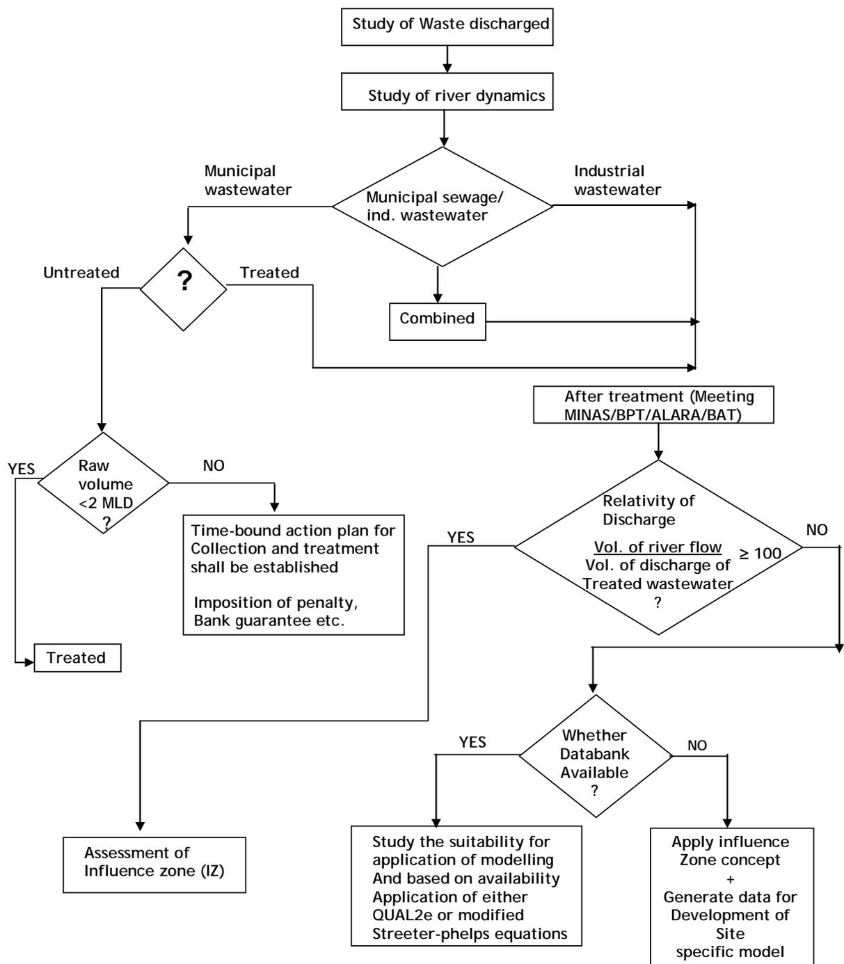
Figure 6.2: Steps involved in the study of River Dynamics and Assessment of its Assimilative Capacity
