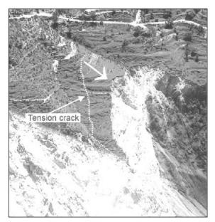
Figure 1: A cracked slope in unweathered Precambrian dolomite at Mukree. Here a block about 50 m in length is sliding forward. At the time of the photograph the tension crack was about 50 cm in width.
