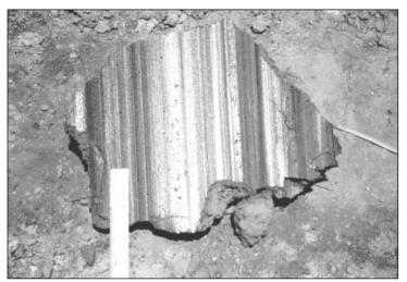
Figure 21: An excellent example of the striated and highly polished and slicken-sided slip surface observed in the undisturbed sample from the basal slip surface of the Watawala Earthslide in Sri Lanka. (Courtesy: R. K. Bhandari)
