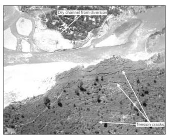
**Figure 2**: A cracked slope in unweathered Precambrian dolomite above the Nisar camp upstream on the Neelum river from Muza arabad. The cracks daylight on a reverse slope at the top of a 200 m cliff. A large failure here during the earthquake blo cked the river, causing the labeled change in the drainage.
