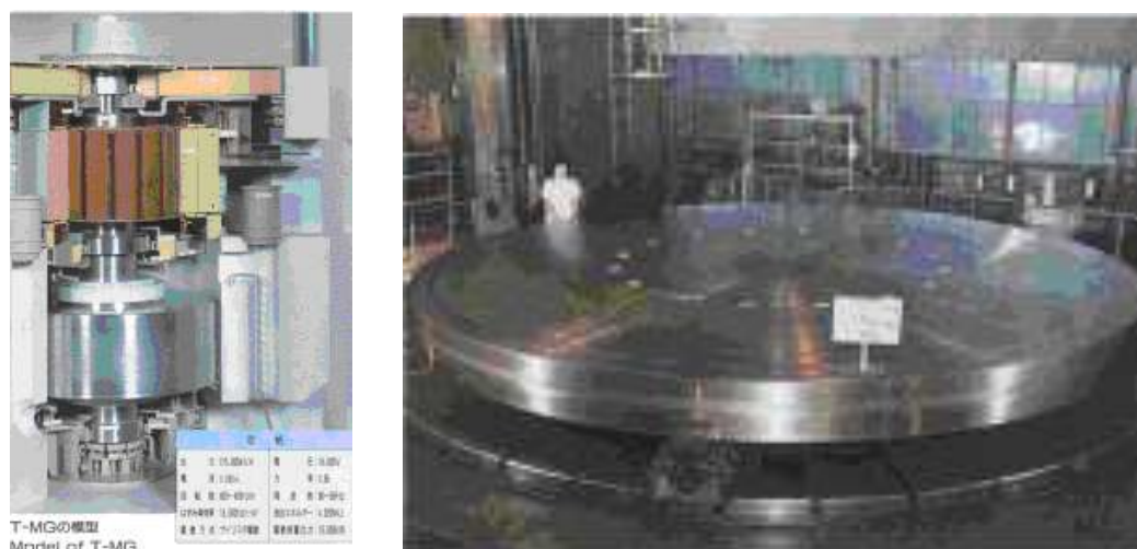
Figure A.47 (left): Cut-away model of the system Figure A.48 (right): Photo of world's largest flywheel
