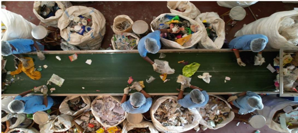
MRF Plant-33 TPD Capacity-Udupi CMC, Udupi Dt
